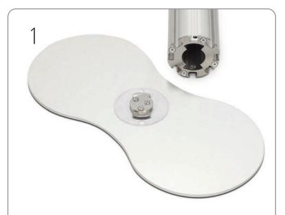
Place base plates on the floor, position lower posts centrally over male fitting of base plate (A), and rotate until assembly drops into position, continue rotating clockwise through 90° to secure (B).
