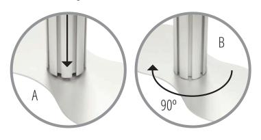
Affix upper posts to lower posts by positioning female end centrally over male fitting (C), and rotate until assembly drops into position, continue rotating clockwise through 90° to secure (D).
