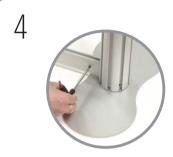
Slot clamps of assembled profile into post channels and tighten grub screws with hex key supplied to secure.
