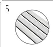
Assemble 950mm vertical profiles in the same way as 750mm profiles, ensuring the steel fixing strips are aligned.
