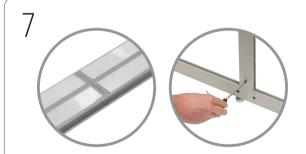
Clamp the middle vertical rails with twin steel fixing strips, halfway across the joins of 750mm bottom horizontal profiles.
