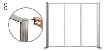
Link final 750mm horizontal profiles, and with the steel strip uppermost, slot onto top of vertical rails and channel of posts. Tighten remaining grub screws to finish assembly of the framework.
