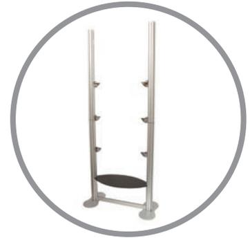
With the black acrylic uppermost, slide first assembly into the same post channels as the bottom profile, until the expanding clamps rest on the pre-installed locator bars of the bottom posts. Tighten grub screws in ends of profile to secure in position.
