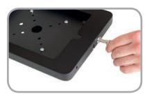
1. Unlock the iPad enclosure by inserting key into security lock and rotate 'QUARTER TURN ONLY' clockwise or counter-clockwise through 90 degrees which releases the locking pin. Return key back to original position to remove and lift fascia out of enclosure.
